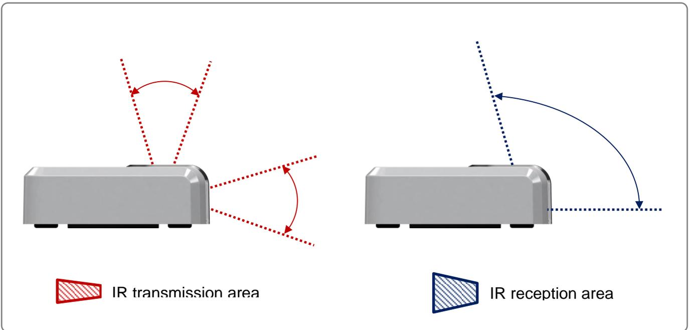
Figure 4-8 IR emitters and IR receiver location
