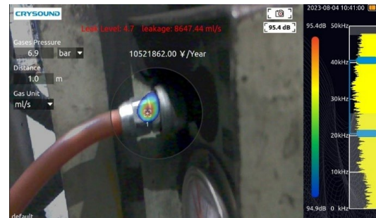
Camera-based air leak inspection
