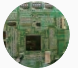
3 DC inverter control
