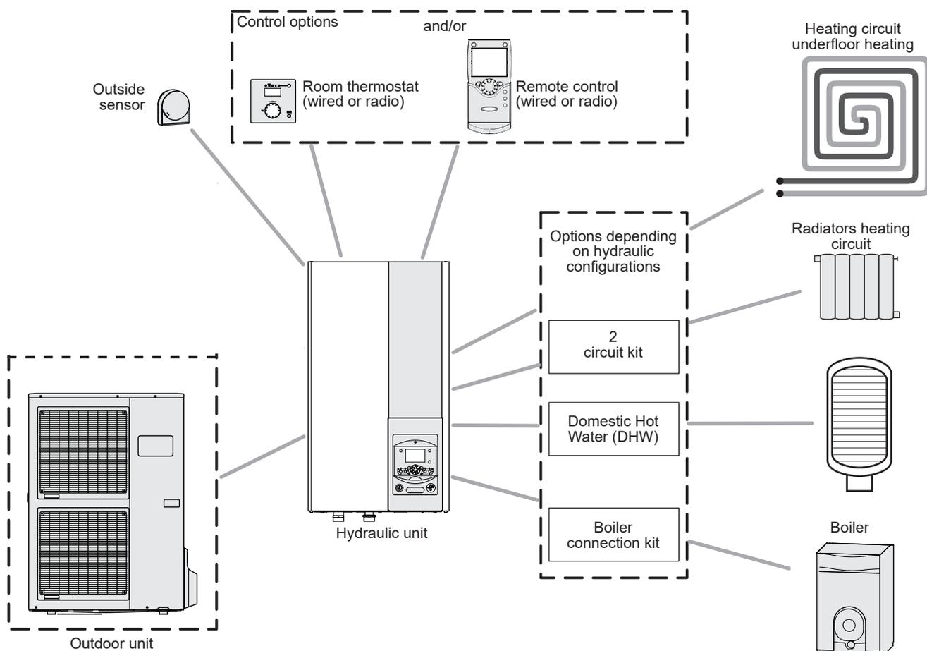
fig. 1 - Overview of complete installation configuration
