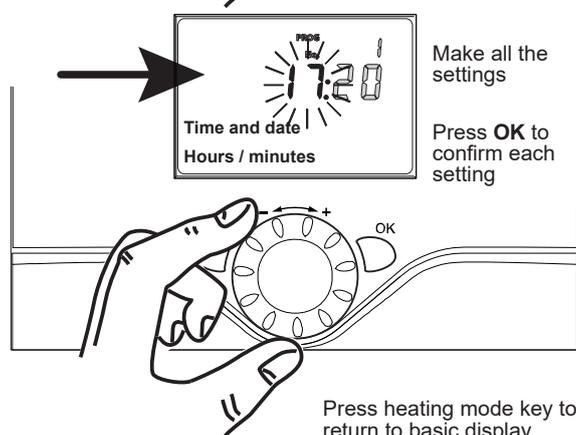
Press heating mode key to return to basic display
